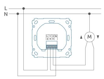
For installation, a neutral conductor is required.
