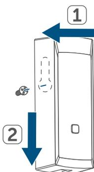
Put the cover (B) onto the electronics unit (D), ensuring that it latches fully into place.
