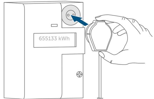
The integrated magnet ensures it remains in place. With standard-compliant interfaces, the cable is routed downwards.
