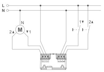
For installation, a neutral conductor is required.
