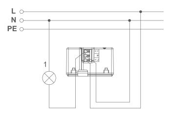
A neutral conductor is required for installation
